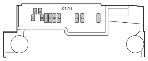
Figure 3. Bottom connector pads in BS8 module
