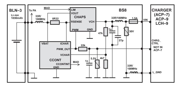
Figure 12. Charging block diagram
