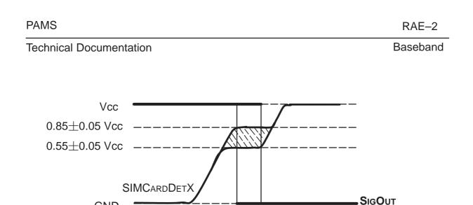
Figure 11. SIMCardDetX detection levels
