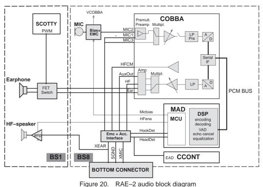
The baseband supports three microphone inputs and two earphone outputs. The inputs can be taken from an internal microphone, a headset mi-
