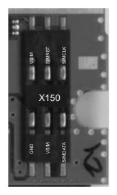
Figure 6. SIM Card Connector
