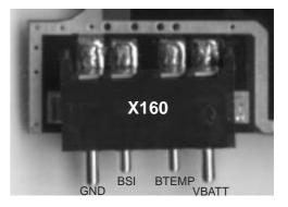
Figure 5. Battery Connector
