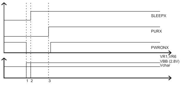
1:Power switch pressed ==> Digital voltages on in CCONT (VBB)
