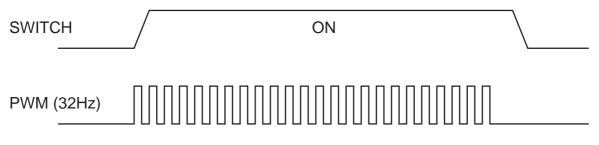
Figure 14. Switch control with 32 Hz frequency (in this case 50% duty cycle)
