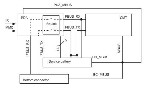
Figure 24. SPOCK's flashing connections
