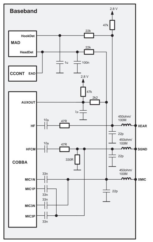
Figure 21. Combined headset and system connector audio signals (Headset can be connected to system connector)
