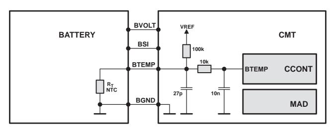
the VREF. The MCU calculates the battery temperature by reading the BTEMP line DC–voltage level with a CCONT A/D–converter.
